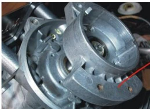
Replacing the magneto once flywheel has been removed to weight.
