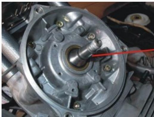
Other side of crank shaft from small pulley. Magneto, coil and flywheel have been removed. A keyway is usually present on this side of the crank. Ensure that the magneto is placed over it in place.
